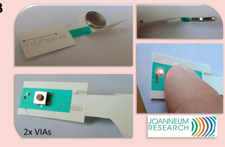
Realization of VIAs: Laser drilling; Filling by dispensing/stencil printing
