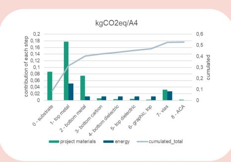
LCA -**Process** flow for twosided electronic paper
