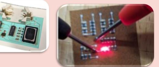
**Assembly** of components using isotropic/anisotropic adhesives
