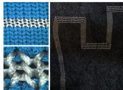
Figure 2: Directly knit stitched wires
