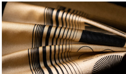
Figure 3: Printed conductive lines
