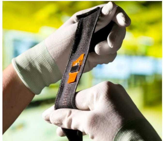
Flexible sensor patch for integration into textiles. ©Fraunhofer EMFT/Bernd Müller
