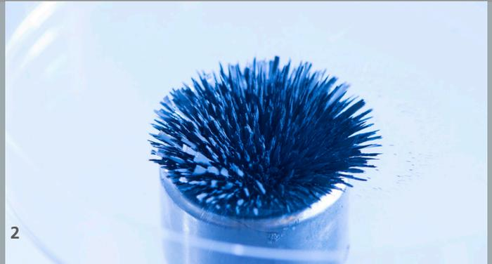
1 | 2 In a magnetic field, the MRF develops a fibrous structure, with tangled chains of particles along the field lines
